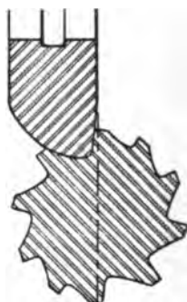
FIG. 49. — FORM OF FLUTE IN REAMER FOR BRASS. TEETH WITH NEGATIVE RAKE, IRREGULARLY SPACED.
